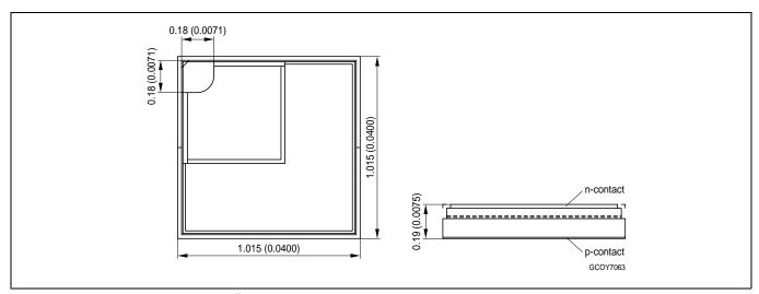
Dimensions are specified as typical<sup>1)</sup> values as follows: mm (inch).
