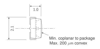
all dimensions in mm. Die placement tolerance  $\pm 0.05.$  Other tolerances  $\pm 0.1$
