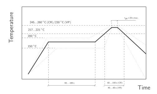
Recommended reflow soldering conditions following IPS/JEDEC J-STD-020.
