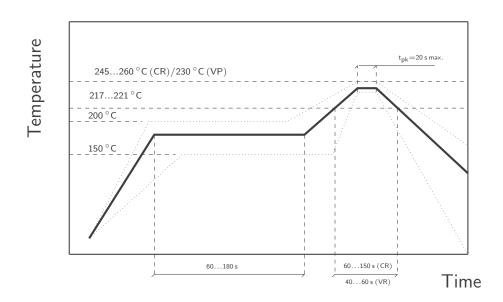
Recommended reflow soldering conditions following IPS/JEDEC J-STD-020.
