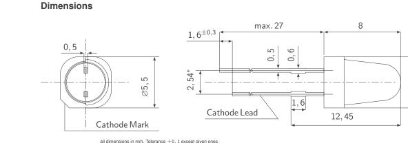
all dimensions in mm. Tolerance  $\pm 0, 1 \mbox{ except given ones}$  at the bottom of the LED
