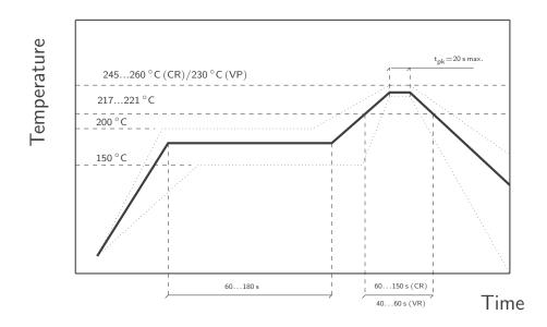
Recommended reflow soldering conditions following IPS/JEDEC J-STD-020.
