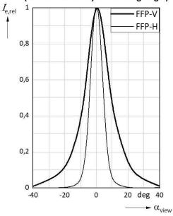
Near Infrared (830 nm) Singlemode Laser Diode
