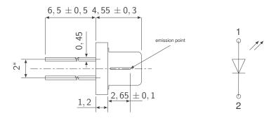
all dimensions in mm. Tolerance  $\pm {\rm 0},$  2 except given ones \* at the bottom of the LED
