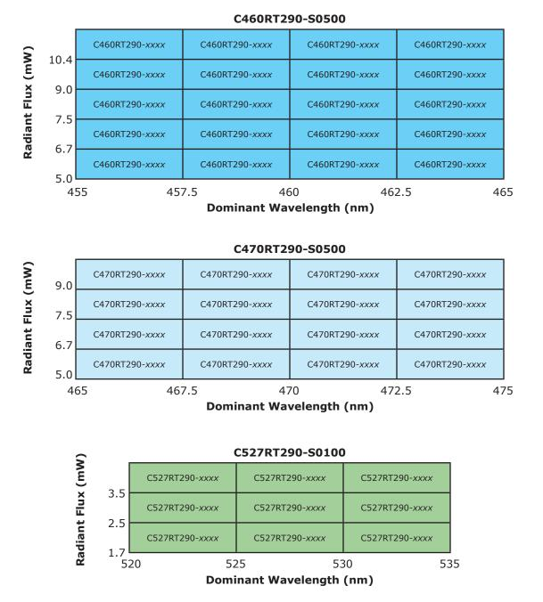
**Note** - Dominant Wavelength shifts shorter with increased forward current ( $I_f$ ). For reference only, the typical DW shift from 5 to 20 mA is -2 nm for Blue LEDs (4xx nm) and -7 nm for Green LEDs (5xx nm).
