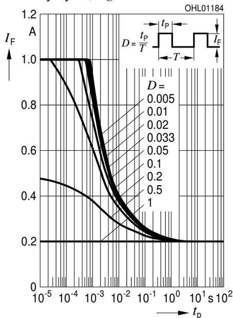
The values shown in the diagrams above, represent the chip in a Advanced Power TOPLED package.
