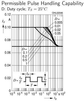
The values shown in the diagrams above, represent the chip in a Power TOPLED package.
