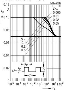
The values shown in the diagrams above, represent the chip in a Power TOPLED package.
