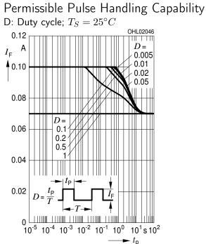
The values shown in the diagrams above, represent the chip in a Power TOPLED package.
