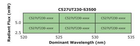
**Note -** Dominant Wavelength shifts shorter with increased forward current  $(I_f)$ . For reference only, the typical DW shift from 5 to 20 mA is -2 nm for Blue LEDs (4xx nm) and -7 nm for Green LEDs (5xx nm).
