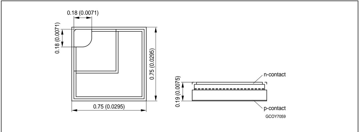
Dimensions are specified as typical<sup>1)</sup> values as follows: mm (inch).
