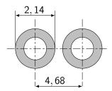
all dimensions in mm. Tolerance  $\pm 0, 1 \; \text{except given ones}$
