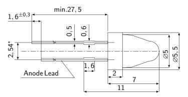
all dimensions in mm. Tolerance  $\pm 0,1$  except given ones  $^*$  at the bottom of the LED
